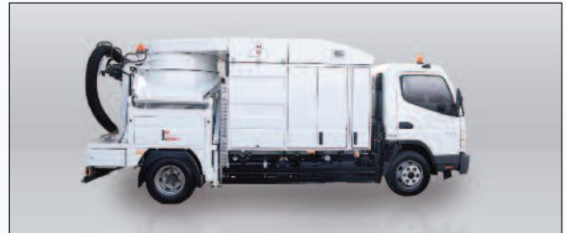
Brechley have been using a number of larger Suction Excavators for over two years on this SEC street light replacement PFI where digging down on live cables is a highly dangerous task; Brechley risk-assessed and found that by using suction excavation, their strike rate fell from one in every 142 mains/disconnection holes dug by traditional means (hand or small tools) down to one in every 546 holes using suction excavation.
